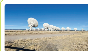
JVLA is an observatory consisting of a total of 27 antennas with an aperture of 25 m. As they were operated in the most compact D formation during my visit, I was able to capture photos of more of those antennas than usual in close range.
