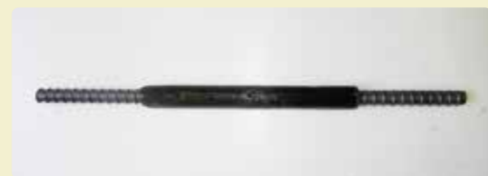
The carbon fibre reinforced plastic sleeve (black inner part) which is used to bond the inner steel bars to one another. The sleeve and the epoxy resin ensure a sturdy bond. The sleeve is incredibly strong, if a pulling force is applied to both sides of the joint, the uncovered steel bar will break long before the sleeve will.
