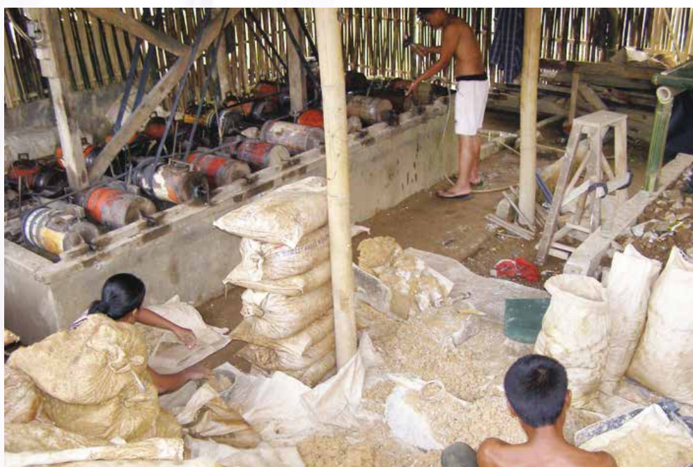
The work place of ASGM. Mercury and crushed gold ore are put in the drums and rotated for several days to extract gold into mercury.
